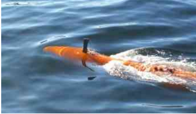
Kongsberg Maritime's HUGIN AUV is a Powerful tool for deep-water hydrographic surveys
