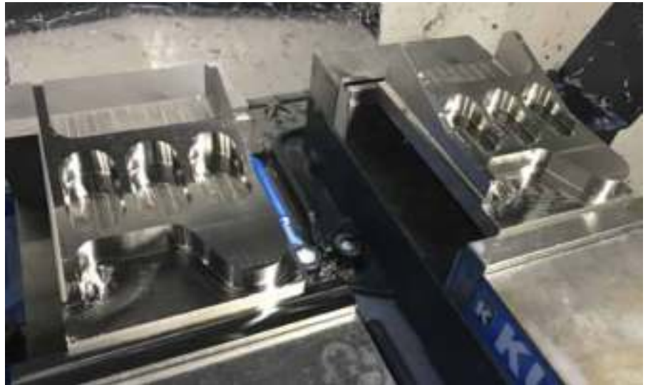
In the Okuma demonstration, the VERICUT Force Optimized finished part on the left was produced more than 20% faster than the original programmed part on the right.
